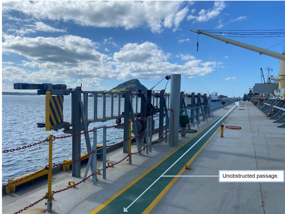
Figure 19: Example of an unobstructed passage.
