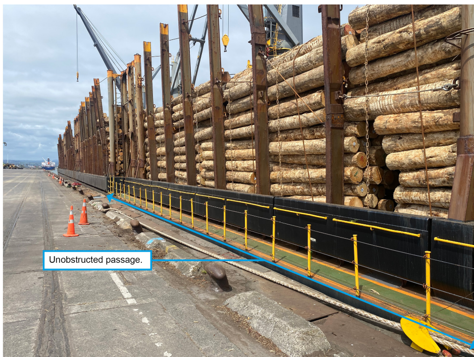
Figure 20: Example of an unobstructed passage.
