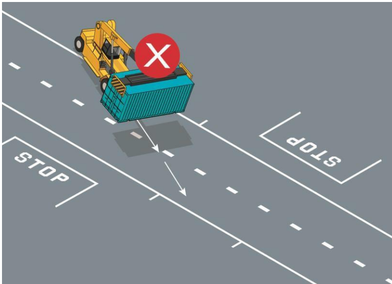
Figure 3 - Shall not cross the common user roadway on an angle or outside the dedicated crossing points.
