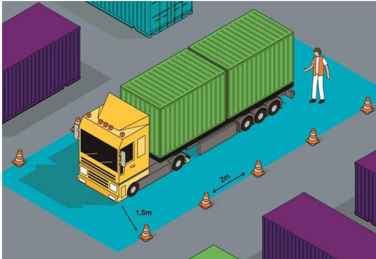
Figure 7 - Example of a temporary DSZ setup by PCBU.
