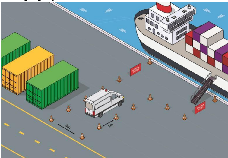
Figure 10 - Delineated Gangway Access
