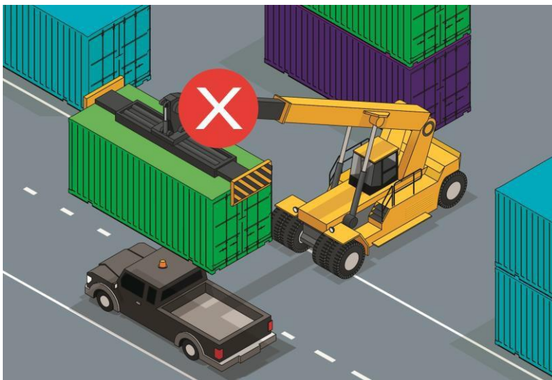
Figure 4 - Loads must not overhang the roadway.
