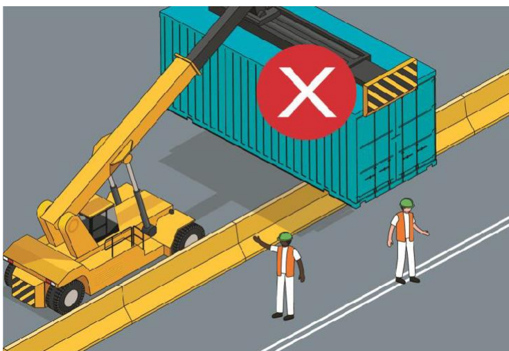
Figure 9 - A load must not protrude over barrier or into other work areas.
