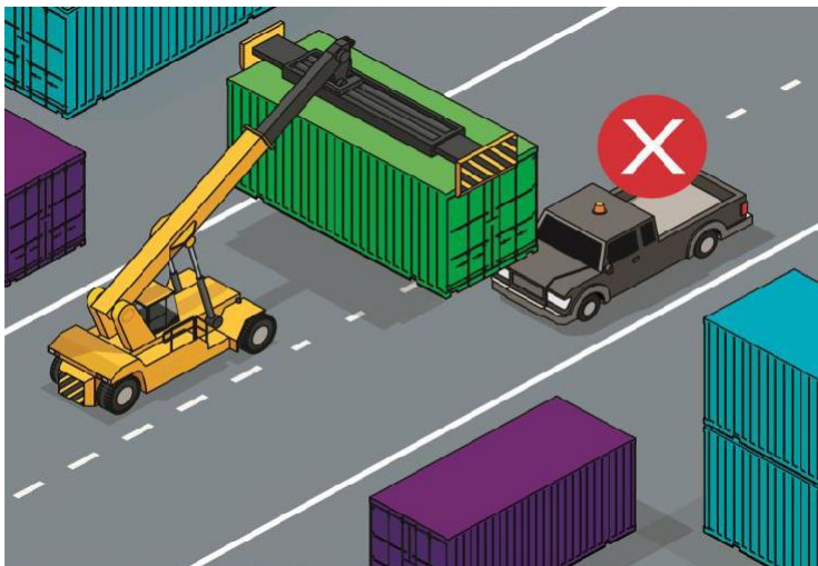
Figure 8 - A load is not to pass over the top of any vehicle.
