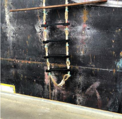
Increased risk of pilot ladder catching on pilot boat. Loop under bottom step not permitted.
